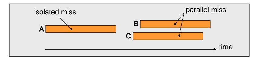
Memory Level Parallelism (MLP) means generating and servicing multiple memory accesses in parallel [Glew' 98]
